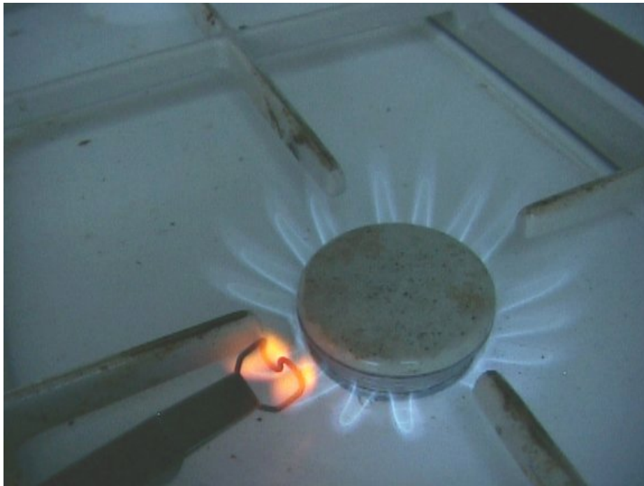
Figure 9: Heat the landmark template while holding it with a pair of pliers until it is red hot.
