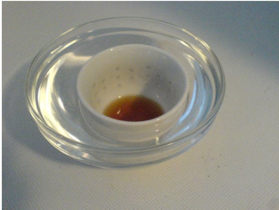
Figure 1: Heat a cup with linseed oil in a bain-marie.
